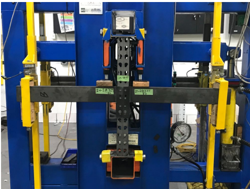
Figure B2-1: Specimen Setup (before test)
