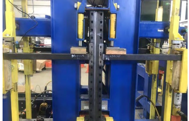
Figure 3 Typical SMHE rack connection test setup
